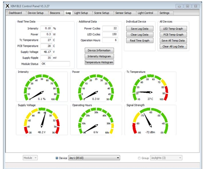
Xicato XIM tracks and reports many operating parameters, and stores internally its operating hours and histograms of its lifetime temperature and intensity. Users can perform proactive maintenance, and Xicato can verify compliance with its warranty.
