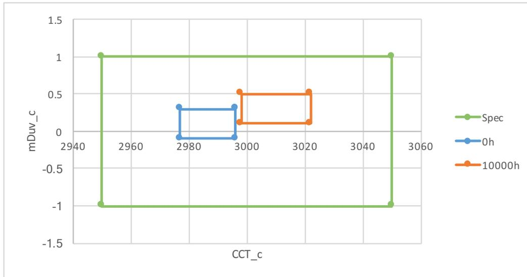
*Xicato color change in both CCT and Duv at maximum current and temperature over 10khrs of entire population of tested units. LM80 testing 2016 by BAACL (Bay Area Compliance Laboratory). Notice that even after 10khrs, all of the modules were still well within Xicato's initial 1x2 MacAdam ellipse specification, and all moved in the same direction.*
