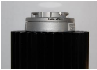
XSM is correctly mounted. The bottom surface of the module is completely flush with the top surface of the heatsink.
