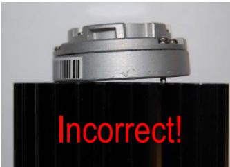
XSM is incorrectly mounted with a gap between the bottom surface of the module and the top surface of the heatsink.
