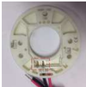
Figure 2: Electrical contacts on the bottom of the housing
