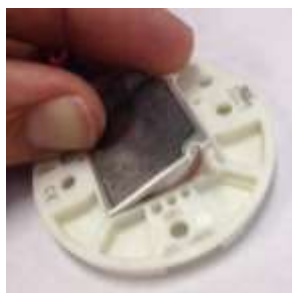
Figure 5: Misaligned XCA Core
