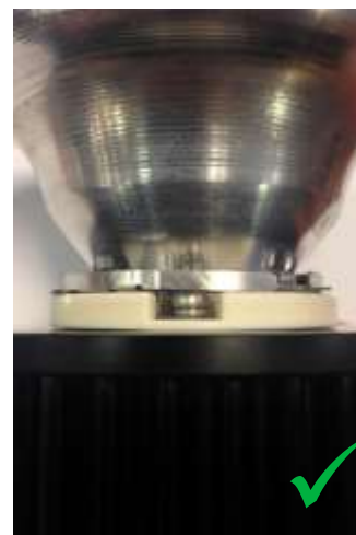
Figure 9: XTM is correctly mounted. The bottom surface of the thermal pad is completely flush with the top surface of the heatsink. Additionally, the screw head, lock washer, and adapter ring flange fit inside the pocket (3.8mm depth) which allows the reflector to sit flush to the optics plane.
