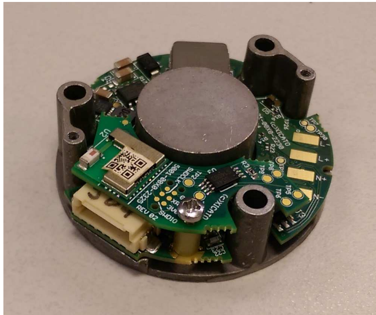
PHOTO 13: PCBs assembled to Thermal Base
