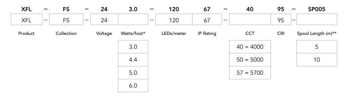
\* 1 Watt/foot = 3.28 Watts/meter
