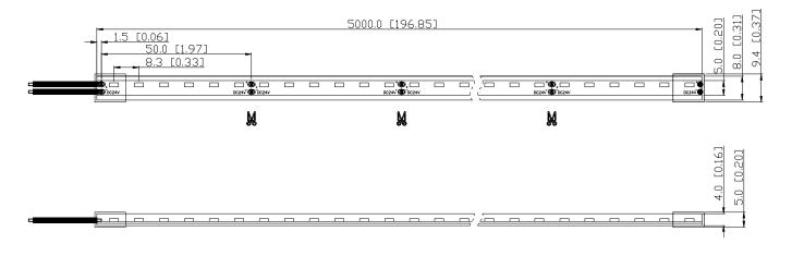
Units: mm (inches) Note: Tolerance ± 0.5 mm
