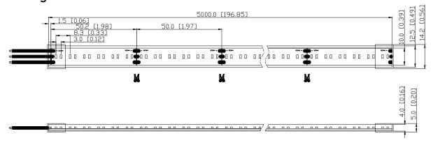
Units: mm (inches) Note: Tolerance ± 0.5 mm
