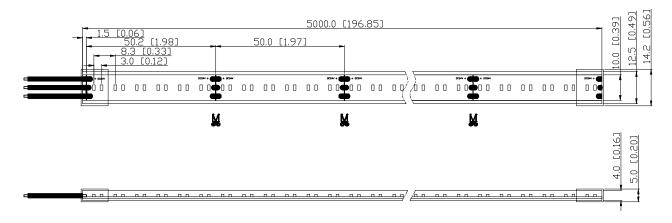
Units: mm (inches) Note: Tolerance ± 0.5 mm Max Bending Radius: Rmin = 20mm
