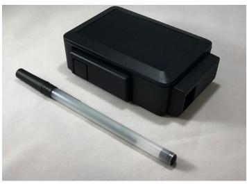
Xicato Intelligent Gateway (XIG-0101) provides range extension, remote monitoring, configuration and control access, and protocol conversion between Bluetooth and IP based protocols such as HTTP and Medialon.
