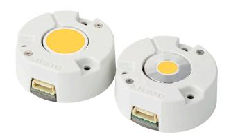
XIM is available in 19mm and 9mm LES, in multiple spectral/CRI formulas and CCTs, and lumen output from 700LM to 3000LM, with Bluetooth®, DALI, and/or 1-10V control.
