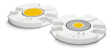
The Xicato Thin Module (XTM) consists of a Xicato Core Array (XCA), pressure fit into a compact yet robust holder designed to allow attachment of a large ecosystem of lenses and heatsinks to facilitate design and construction of a wide variety of downlight and spot fixtures.
