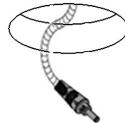
Low Voltage Wiring to XDL Downlight
