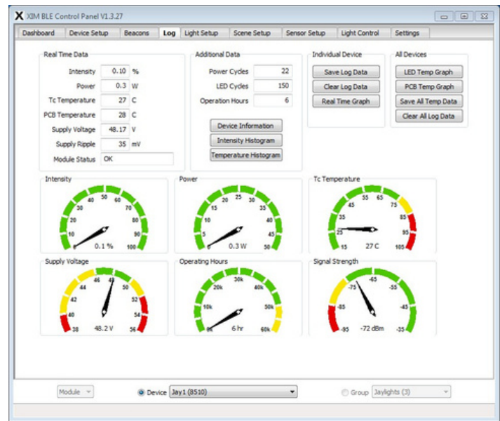
Control Panel log screen, showing real-time operational data
